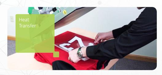
Images are printed onto specialised heat transfer paper using a laser printer and transferred to the garment using a heat process. The process supports local production and personalisation (like Inkjet DTG) but can be fiddly as images must be printed in reverse, the heat transfer paper has to be trimmed before the image is applied and specialised paper is required to apply a white underlay.
