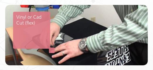
Vinyl or Cad Cut printing also uses a similar process to heat transfer. Designs (logos, shapes, letters and numbers) are cut from a special vinyl material using an industrial cutting machine or plotter and transferred to garments using a heat press. The process is ideal for printing one or two-colour messages or logos onto garments.
