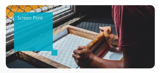
This is a high volume print process. A blade or squeegee presses inks through a mesh stencil or screen onto the garment. Each colour requires a separate screen which must be accurately aligned to ensure registration. As the screen rebounds away from the substrate the ink remains on the substrate. Textile printed with multi-coloured designs use a wet on wet technique.
