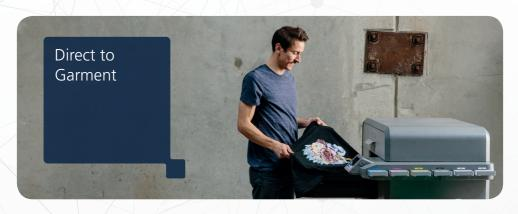
DTG (Direct to Garment) is a relatively new garment printing technology. It uses purpose designed inkjet printers, such as Ricoh's Ri 3000 and Ri 6000, to apply water-based pigment inks directly to cotton and cotton/polyester mix garments. Because the process is digital, the design can be changed from one garment to the next.
